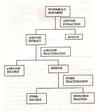
Figure 1. Schematic fractionation of acetone extract
