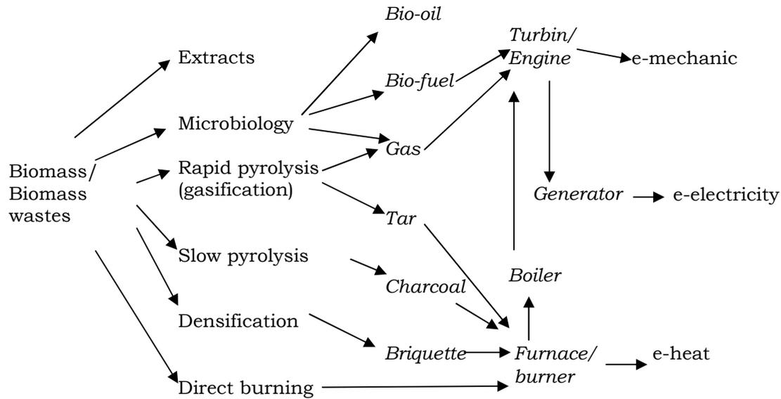
**Figure 2.5.** Technology choices for conversion of biomass/biomass wastes to energy
